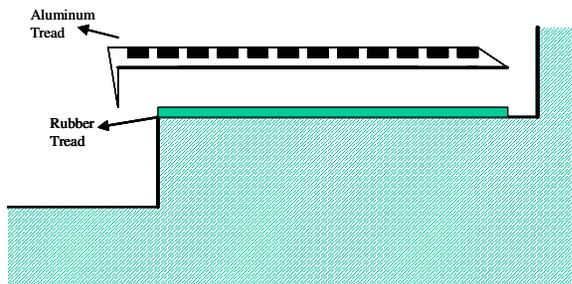
**IMPORTANT:** Only drill into the existing holes on the perimeter of the Aluminum tread. Doing otherwise may cause damage to the heating elements inside the mat. Use 3/16 x 2” screws that are appropriate for the stair surface (i.e. wood, cement, steel).
