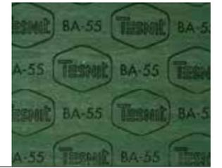
**GASKET MATERIAL WITH EXCELLENT THERMAL PROPERTIES AND GOOD STEAM RESISTANCE**
